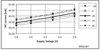
Figure 20. DC current vs. supply voltage, mode = high
